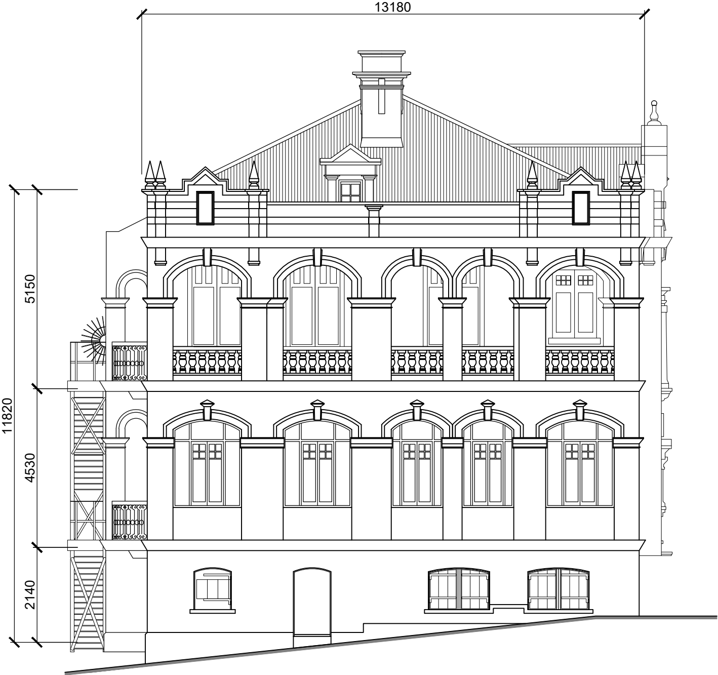
1 NORTHWEST ELEVATION MAIN BLOCK
