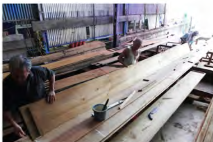
本土工匠為香港大澳傳統龍舟協會製作龍舟，他們正安裝船底大勝，俗稱「上大勝」的工序。 Local craftsmen set the garboard strakes for a dragon boat built for the Joint Association of Traditional Dragon-Boats in Tai O, Hong Kong.
